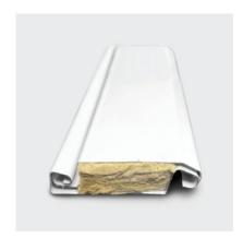
**SLAT PROFILE**: Manufactured from commercial-grade galvanized steel and coated with super durable polyester paint backed by a 40-year film integrity and 25-year no-fade paint warranty. Mineral wool thermal insulation, effective insulating value to be R=4.7.
