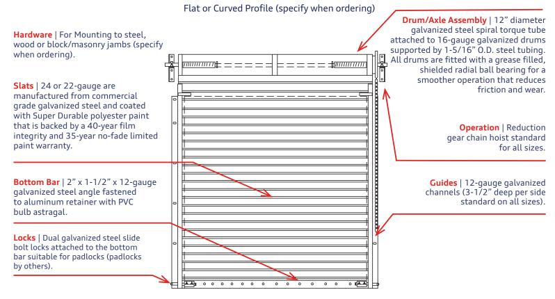
The 300 Series Commercial Slat Door with nylon end locks and 12-gauge roll formed guides is an economical alternative slat door that is easy to maintain and service. The curtain is pre-assembled on the drum at the factory making the installation easier and faster.
