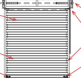
Drum/Axle Assembly | 12" diameter galvanized steel spiral torque tube attached to 16-gauge galvanized drums, supported by 15/16" O.D. steel tubing. All drums are fitted with grease filled, shielded radial ball bearing for smoother operation, reduced friction and wear.
