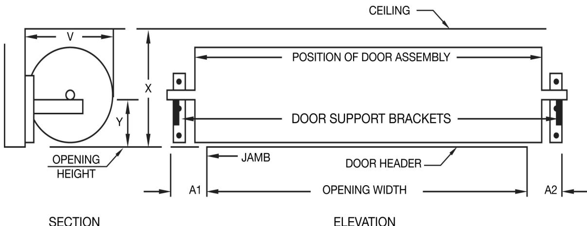
**CEILING: LOCATE DIMENSIONS AND CLEARANCE ON DIMENSION PANEL. STANDING ON THE INSIDE FACING OUT. DRIVE TYPE IS ON RIGHT SIDE UNLESS OTHERWISE SPECIFIED.**
