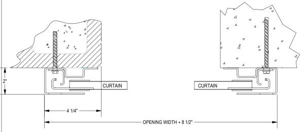
FIGURE 13: CONCRETE / MASONRY JAMBS
