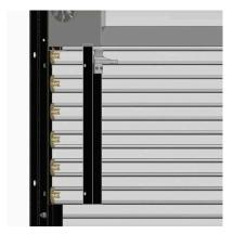
**GUIDES:** Angles to be 3/16" minimum thickness structural steel with removable head stops and 30" service cut-out. Guide depth to provide slat penetration adequate to satisfy specified windloading.
